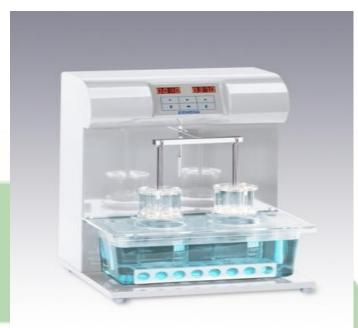
On the ZT 222 series (available 1 to 4 test stations, operating simultaneously) the counting of the elapsed test duration is automatically started/ stopped the arm with the basket is lowered/raised manually.
