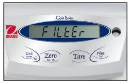
To help adapt the balance to real life working conditions, the PAJ is designed with selectable environmental settings. When working in harsh environments, the balance can be adjusted to compensate for vibrations and other disturbances. Conversely, the balance can be adjusted for working in slow filling applications where sensitivity is a must.
